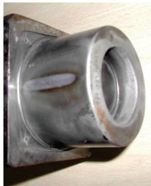
Fig. 1.1 Moving Core of the Die showing high wear near the gate area.
